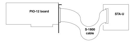
Figure 1. Connecting the PIO-12 Board to an STA-U
